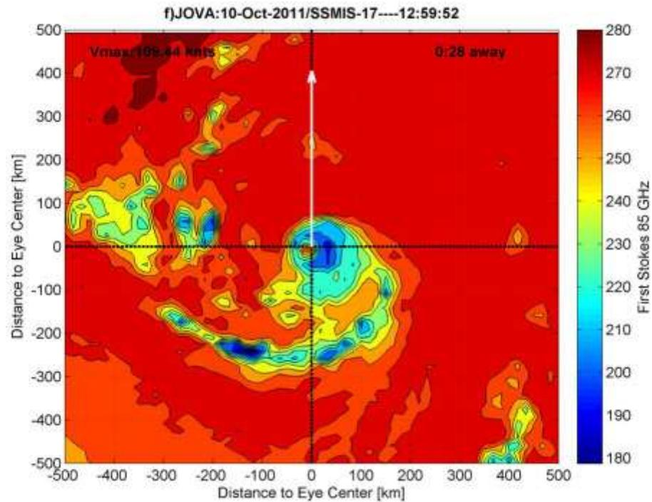
SMOS Tb is rotated to a fixed "North up" propagation direction for further averaging of Tb
