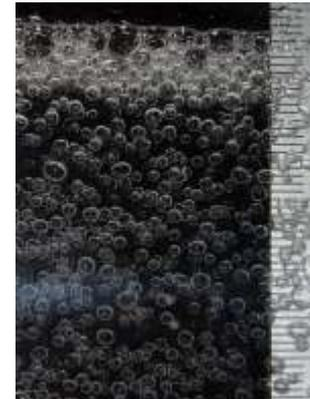
Empirical measurements made before the launch of SMOS to assess the impact of ocean foam on the L-band signal
