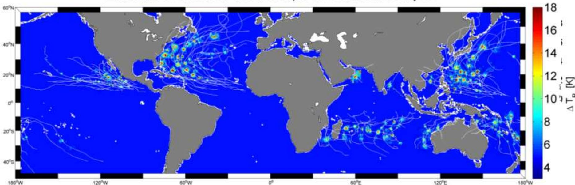
A subset of 320 SMOS swath intercepts with TCs over 2010-2015, free of Radio Frequency Interferences and with pixel distances >150 km from coasts are selected
