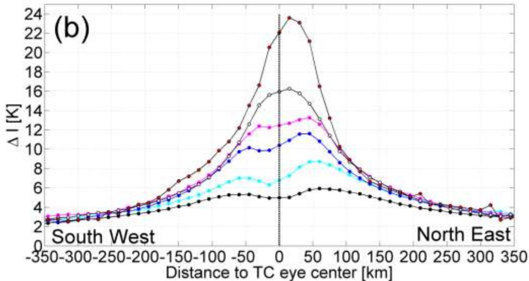
SMOS surface Tb data reveal a clear average growth of amplitude with storm intensity
