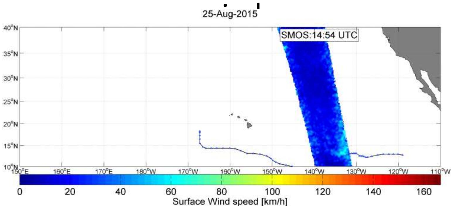
A time-series mosaic of surface wind speed measurements from 25 Aug to 8 Sep 2015 over Hurricanes Kilo, Ignacio and Jimena is shown in this animation. Data from three satellite microwave radiometer missions: the ESA L-band SMOS mission, the recently launched NASA L-band SMAP mission and JAXA C-band AMSR-2 mission are combined before your eyes to reveal the track of each Hurricane and the maximum surface wind speed.
