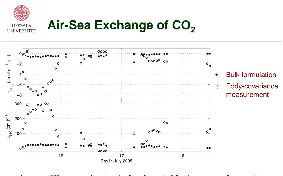
Large difference is due to **horizontal heteorogenity** and **sea surface measurements not being in the flux footprint area**.
