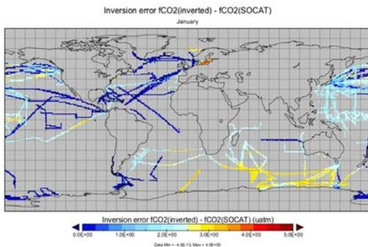
Figure 5. Calculated 'inversion error' in  $f_{CO_2,cl}$  estimated for January 2010; on a 0 to 5  $\mu\text{atm}$  scale.
