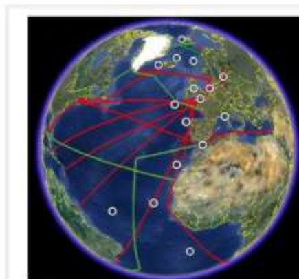
Fig. 1: The suggested network of stations for the ocean-network Circles - Fixed Ocean Stations (FOS), Red lines - Voluntary Observing Ships (VOS), and green lines - Repeat Ocean Sections (ROS).
